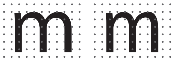
Figure 5.6: Stem adjustment. An untouched m and a stem adjusted m . Note that for a monochrome rasterizer, these could use some dropout control for the arcs as well, as they are completely missed by the pixel centers and therefore cause gaps.
